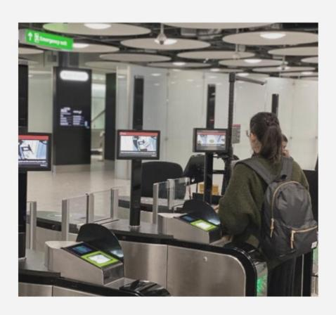
At Heathrow T2 and T5, all domestic travellers are required to enrol in the Aurora Face Recognition system as they transit airside. When they present their boarding pass at the entry to security checks (ticket presentation), the data on the barcode is checked and if they are travelling to a domestic destination, the face recognition camera starts and they can only proceed once the enrolment is completed.
